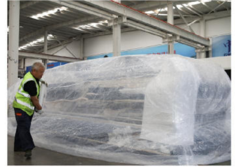
03 Protective Film Wrapping
