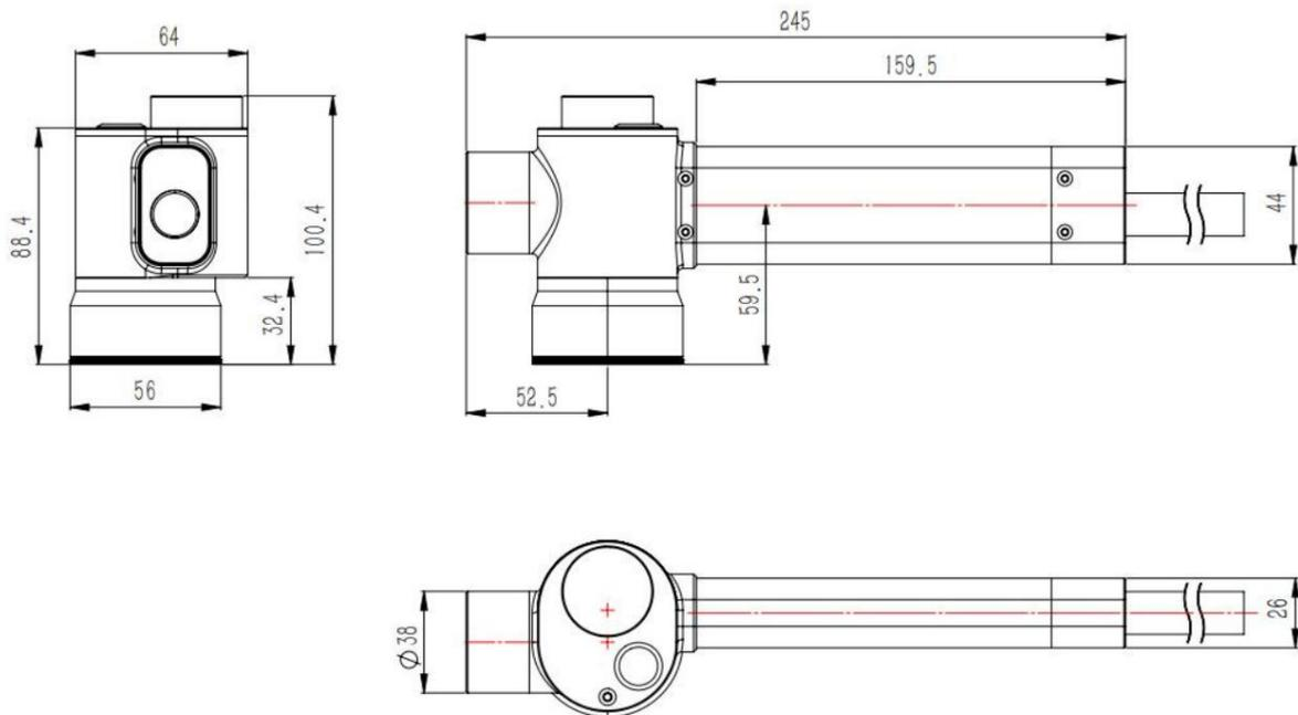
Figure 6 Dimensional diagram of cleaning gun head
