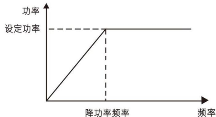
Figure 3 The power reduction frequency corresponds to the output power change
