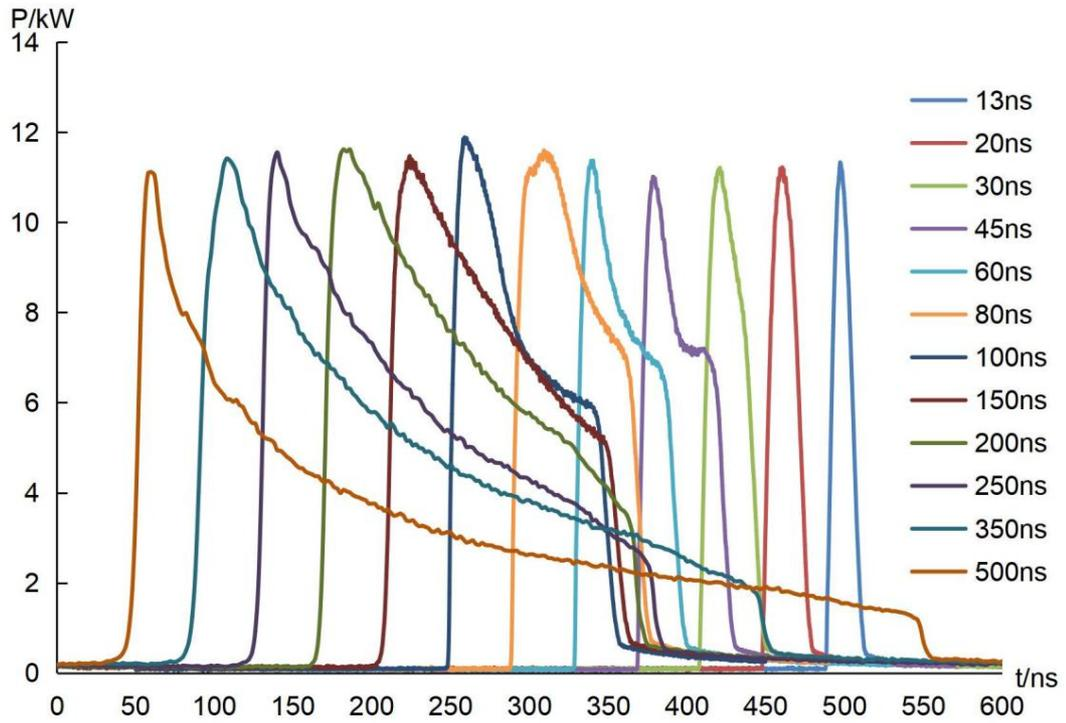
4-1 YDFLP-CL2-200-1-A output waveform curve diagram
