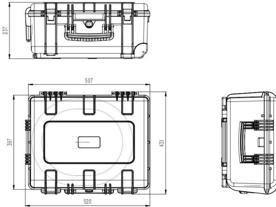
Figure 5 Dimensions of the outer box of the cleaning machine
