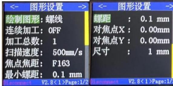
Figure 18.2 Parameters of Archimedes spiral
