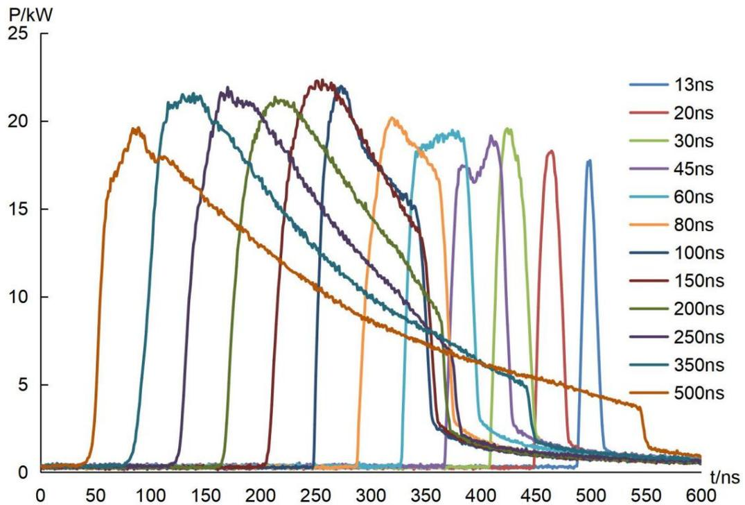
Figure 4-2 YDFLP-CL2-200-5-A output waveform curve
